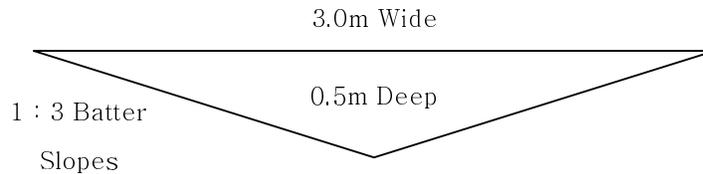
*Figure 3 – Nominated Swale Drain Dimensions*
